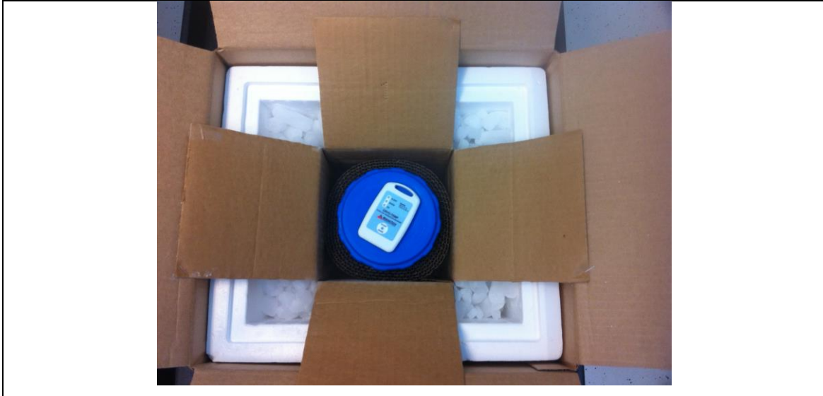
Figure 2: White (Dry Ice) Data logger placement
