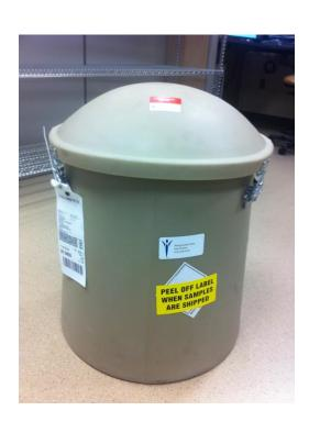
Figure 1: Red Kit (LN<sub>2</sub> dry vapor shipper)
