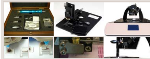
Figure 2: (top) Instruments used for TMA construction: (left) hand-held Quick-Ray (UNITMA Co., Ltd., Seoul, Korea), (center) manual bench top MTA I (Beecher Instruments, Sun Prairie, WI, USA), (right) semi-automatic TMArrayer (Pathology Devices, Westminster, MD, USA). (bottom) All can be used to construct equally useful TMA blocks. Photos courtesy of the manufacturers.
